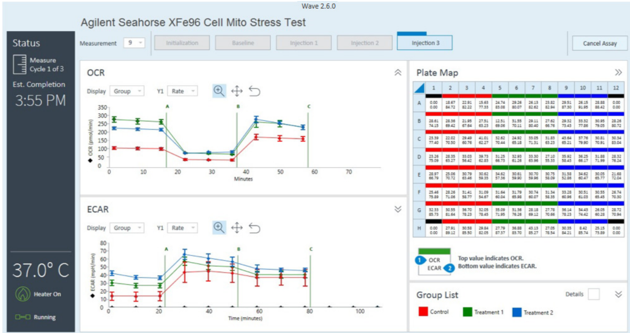
Figure 32 Data acquisition runtime display on an XFe Analyzer
